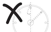
For all grinding, sanding, and wheel type wire brushing accessories, the lowest portion of the accessory must be contained within the guard enclosure with 2 mm or greater clearance to the bottom lip of guard.
