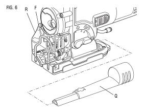
2. Fit the dust extraction adaptor (Q) to the tool as shown.
