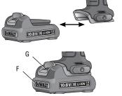
To remove the battery pack from the tool, press the release button (G) and firmly pull the battery pack out of the tool handle. Insert it into the charger as described in the charger section of this manual.
