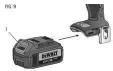
To install the battery pack into the tool handle, align the battery pack with the rails inside the tool's handle and slide it into the handle until the battery pack is firmly seated in the tool and ensure that it does not disengage.
