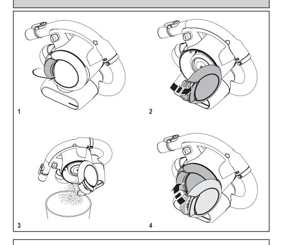
In order to keep the suction force optimised, the filters must be cleared regularly during use.
